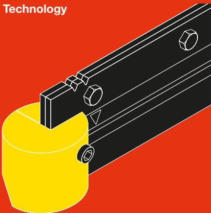
The curbstone deflector is simply screwed to the clearing blade and provides optimum protection for the edges. The blades wear down evenly, considerably extending their durability. The curbstone deflector may be replaced at any time.
